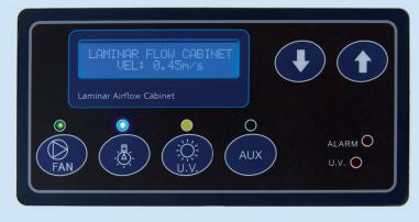
Digital control board with LCD display\* including:
